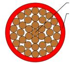
Bare copper conductor Rubber compound insulation
